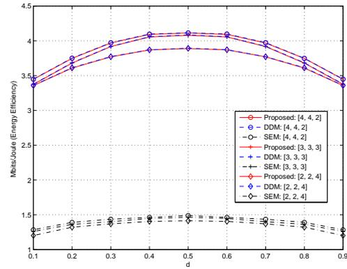
Fig. 2. EE against d where d is the distance between terminal  $T_1$  and relay  $T_3$ . Here  $P_{max} = 5$  Watt,  $\beta = 0.01$ ,  $P_c = 0.5$ , and  $[\alpha_1, \alpha_2, \alpha_3] \in \{[4, 4, 2], [3, 3, 3], [2, 2, 4]\}$ .
