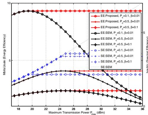
Fig. 4. EE/SE against  $P_{max}$  where  $d = 0.5$ ,  $\beta \in \{0.1, 0.01\}$ ,  $P_c \in \{0.1, 0.5\}$ , and  $[\alpha_1, \alpha_2, \alpha_3] = [3, 3, 3]$ .
