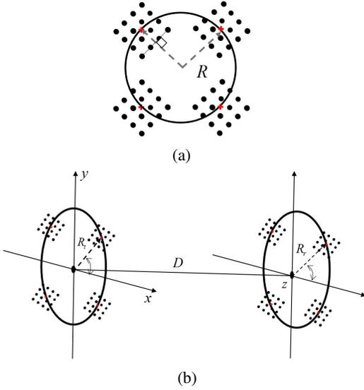
Fig. 1: (a) UCA-SA with  $N_s = M = 4$ . Here  $R$  is either  $R_t$  or  $R_r$ . (b) UCA-SA coordinate system with  $N_s = 4$ .
