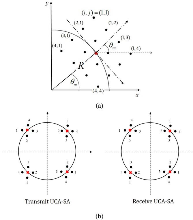
Fig. 3: (a) Coordinates of antenna elements when  $M = 4$ . (b) Decomposition of a UCA-SA system with  $N_s = 4, M = 2$  into four UCA sub-systems. Here antennas with identical indices form a UCA sub-system.
