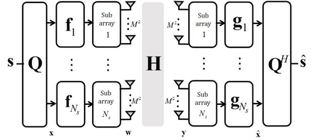
Fig. 2: UCA-SA system. The transmitter employs the beamformer  $\mathbf{F}$  and the DFT precoder  $\mathbf{Q}$ ; the receiver employs the beamformer  $\mathbf{G}^H$  and the IDFT decoder  $\mathbf{Q}^H$
