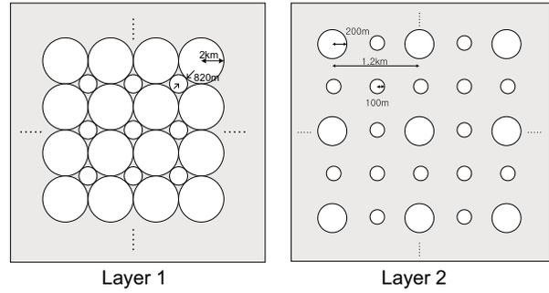
**Figure 3. A CDMA network composed of two cell layers for example 1.**
