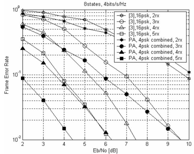
Fig. 5. Frame error rate comparison between 16PSK-8state STBC-MTCM of [3] and PA for 2x2, 3, 4 and 5 MIMO systems
