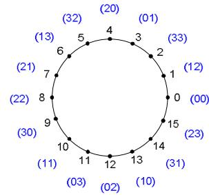
Fig. 3. Description of the mapping of two QPSK signals into 16-PSK for the 8-state QPSK STTC of [12]
