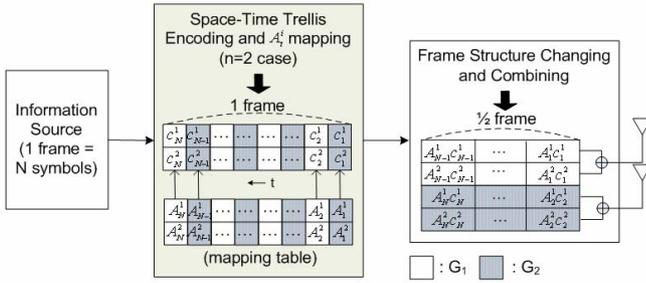
Fig. 4. Block diagram of the transmitter based on the IS-VA approach
