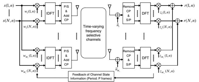
**Figure 1: Block diagram of a MIMO-OFDM system with  $M_t$  transmit antennas,  $M_r$  receive antennas, and  $N$  subcarriers.**
