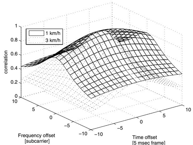
Figure 2: Frequency- and time-domain correlation of beamforming vectors.
