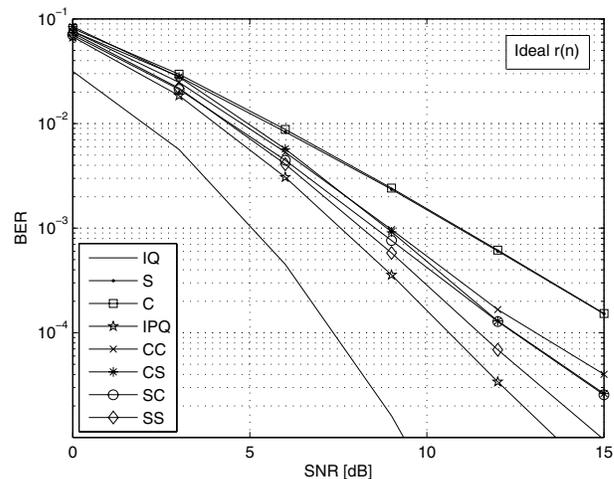
Figure 3: Uncoded BER performances of 1D and 2D beamformer selection schemes in time-varying channels with ideal  $r(n)$ .
