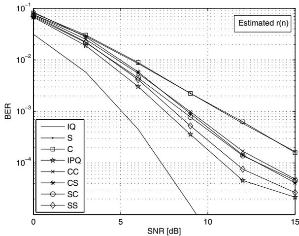
Figure 4: Uncoded BER performances of 1D and 2D beamformer selection schemes in time-varying channels with estimated  $r(n)$ .
