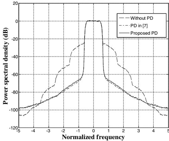
Fig. 4. Comparison of power spectral density at PA output ( $P = 3$ ).
