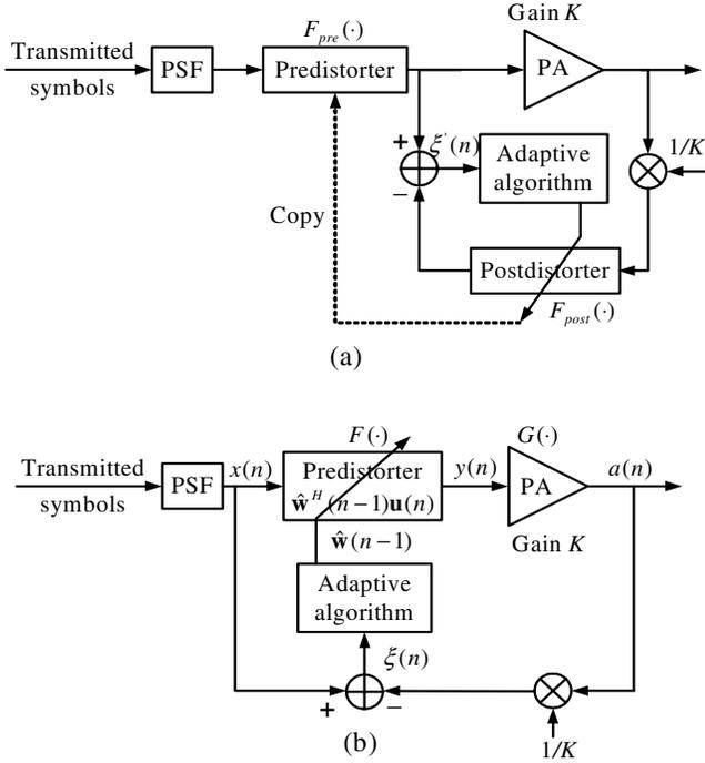
Fig. 1. Transmitter model employing PD. (a) indirect learning architecture [7]–[9] (b) proposed architecture.
