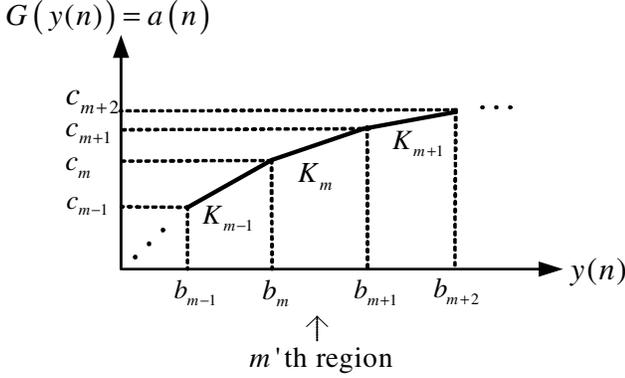
Fig. 2. Piecewise linear model of PA
