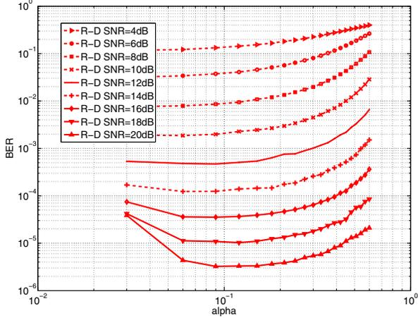
Fig. 5. Coded BER versus  $\alpha$  (R-D SNR = 12 dB).
