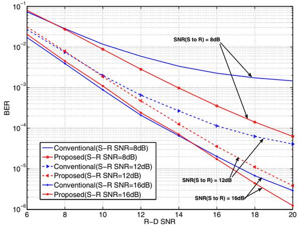
Fig. 6. Coded BER performance (S-R SNR = 8, 12, 16 dB).
