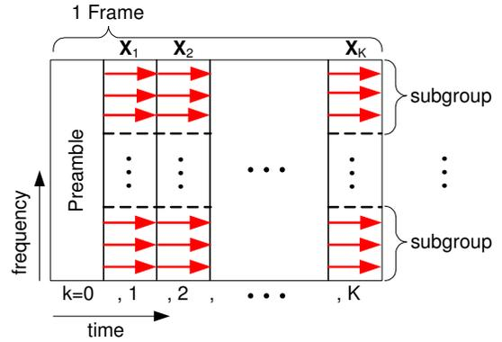
Fig. 2. An OFDM frame consisting of a preamble and  $K$  OFDM symbols, where  $\mathbf{X}_k$  is an OFDM symbol and each subgroup contains  $N_P$  equi-spaced pilots (arrows in the OFDM symbols represent pilot subcarriers).
