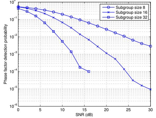
Fig. 3. Phase factor detection error probability under quasi-static fading channels.
