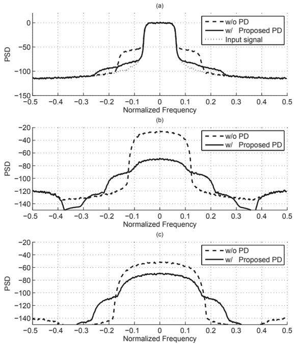
Fig. 6. Power spectral density at PA output. (a) zoom in around  $\omega_o$ , (b) zoom in around  $2\omega_o$ , (c) zoom in around  $3\omega_o$
