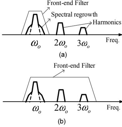
Fig. 1. PA output for (a) single-band system (b) dynamic spectrum allocation system.
