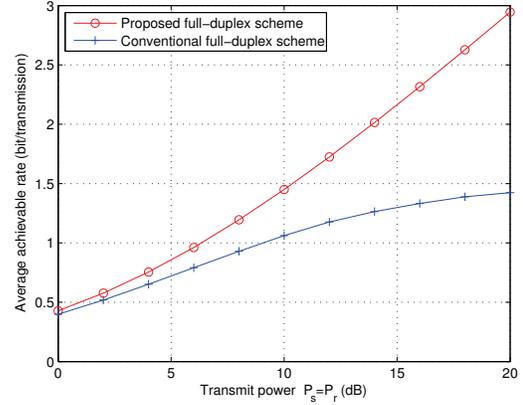
Fig. 2. Average achievable rate of the proposed and the conventional scheme with i.i.d.  $\mathcal{CN}(0, 1)$  channel and  $P_s = P_r$ . Averaged 100 times.
