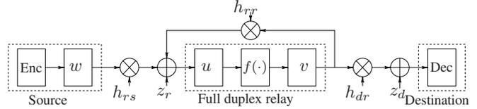
Fig. 1. Block diagram of the considering two-hop decode-and-forward relay system with the self-feedback cancellation.
