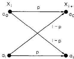
FIG. 5. State Transition Diagram for Binary Symmetric Signal Model.
