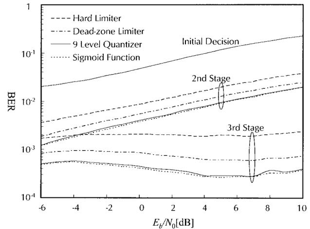
Fig. 6. BER of the users in group 1 when  $E_2 = E_4 = \dots = E_{30} = E_{g1}$  (group 1) and  $E_1 = E_3 = \dots = E_{31} = E_{g2}$  (group 2). The  $E_b/N_o$  for group 1 is set at 10 dB.
