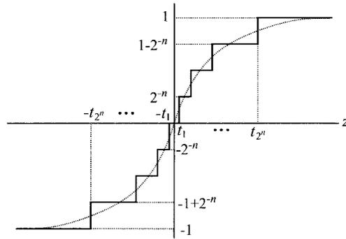
Fig. 3. A multilevel quantizer (the dotted curve shows a sigmoid function).
