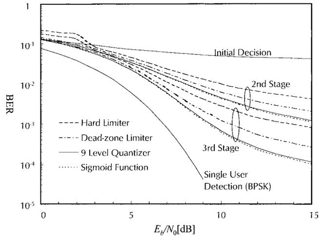
Fig. 5. BER versus  $E_b/N_o$  for 31-user systems when  $E_1 = E_2 = \dots = E_{31}$ .
