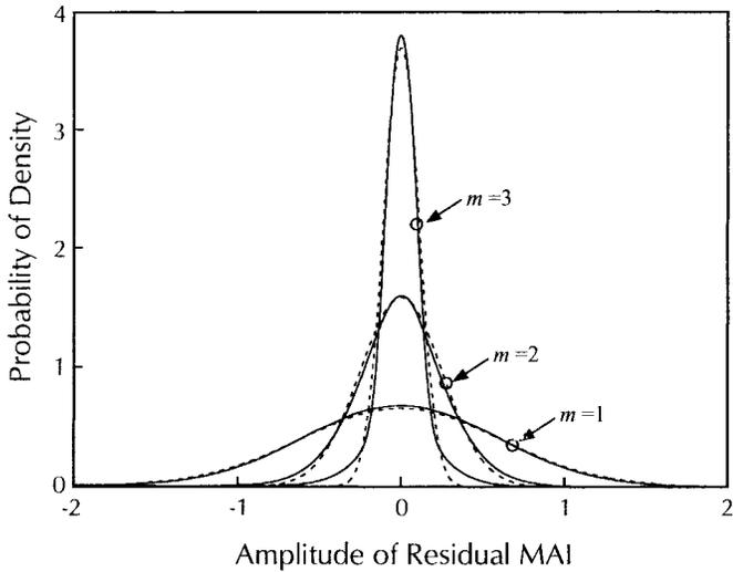
Fig. 4. Comparison between empirically estimated pdf's of the residual MAI in each stage (solid curves) and corresponding Gaussian pdf's (dotted curves). Here, the sigmoid function in (11) is employed,  $E_b/N_o = 8$  dB, and  $M = 3$ .
