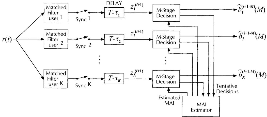
Fig. 1. The multistage detector for the BPSK-CDMA system.
