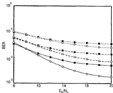
Fig. 3 Comparison of BER values between conventional receiver in Fig. 1 and SAIC in multipath Rayleigh fading channels
