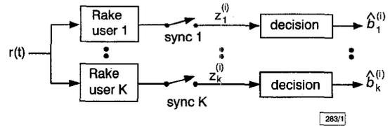
Fig. 1 Conventional detector employing Rake receiver for each user
