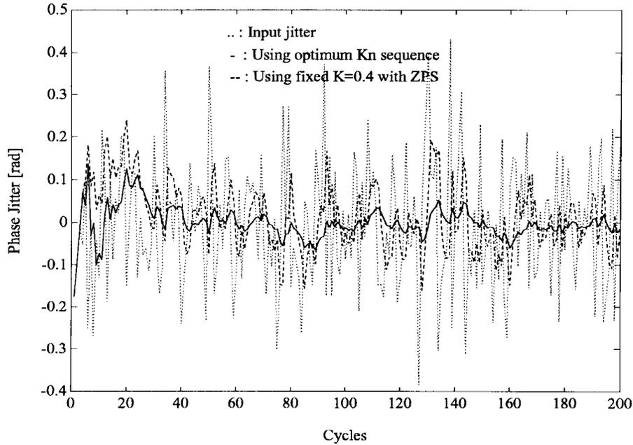
Fig. 7. Real-time phase acquisition using the optimum  $K_n$  sequence and a fixed value of  $K$  ( $= 0.4$ ) where  $\sigma_N^2$  and  $\beta$  are  $0.15^2$  and  $0.95$ , respectively.
