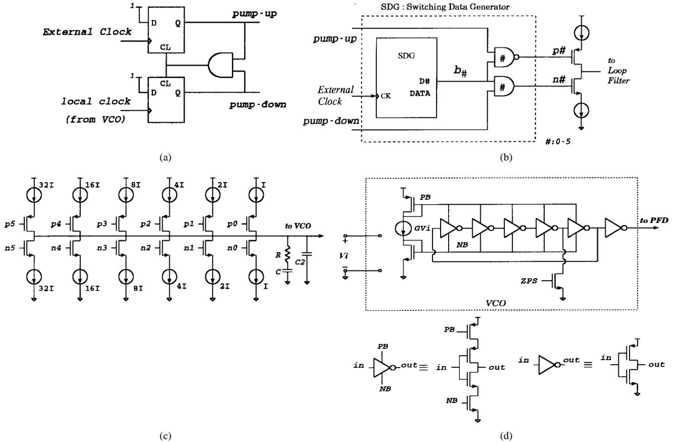
Fig. 11. Simplified schematics of the basic circuit elements. (a) PFD. (b) Gear-shifting control. (c) Charge-pump and loop filter, here  $I = I_{\min}$ . (d) VCO.
