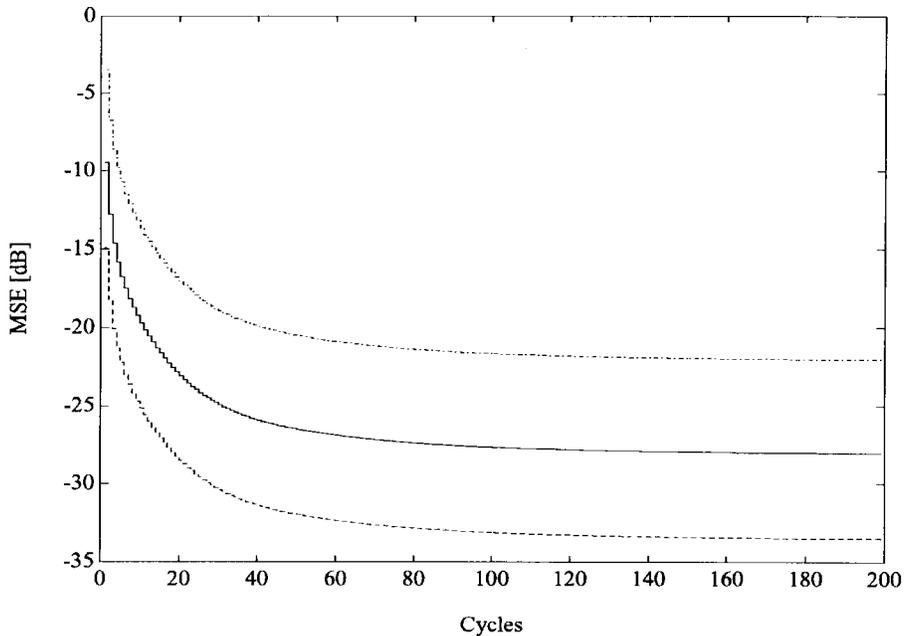
Fig. 5. MSE using optimum  $K_n$  sequence with several noise variances  $\sigma_N^2 = 0.3^2$  (· · · · ·),  $0.15^2$  (—) and  $0.08^2$  (— —), where  $\beta = 0.95$ .
