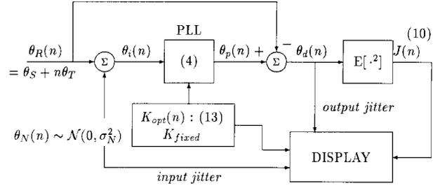
Fig. 3. Simulation setup for the behavioral model of the optimum gear-shifting CP-PLL. Numbers refer to equations.
