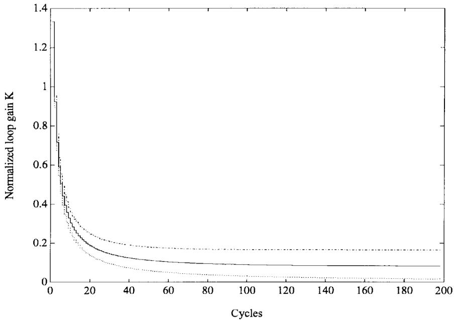
Fig. 4. Optimum gain sequences with various  $\beta$  i.e., 0.9, (· · · · ·), 0.95 (—), and 0.9986 (— —).
