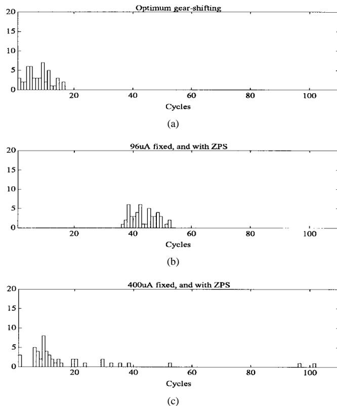
Fig. 15. Histograms illustrating the acquisition speed of the CP-PLL's. The horizontal-axis represents the acquisition speed in cycles, and the vertical-axis is the number of the jitter patterns for which the acquisition is achieved.
