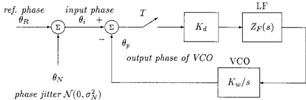
Fig. 1. Linearized model of CP-PLL where  $K_d$  is the gain of the phase frequency detector (PFD),  $Z_F(s)$  is the loop filter transfer function, and  $K_w$  is the VCO gain.
