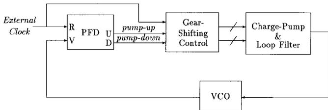
Fig. 10. Block diagram of a gear-shifting CP-PLL.
