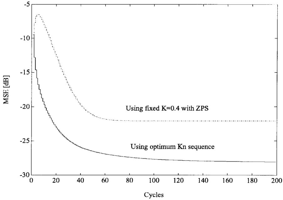
Fig. 6. MSE comparison between the CP-PLL's with the optimum  $K_n$  sequence and a fixed value of  $K$  ( $= 0.4$ ) under conditions of approximately equal convergence rates. Here  $\sigma_N^2 = 0.15^2$  and  $\beta = 0.95$ .
