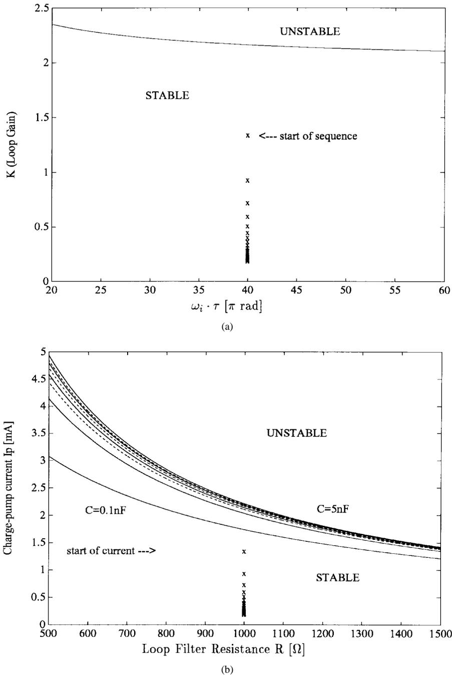
Fig. 12. Stability limit when  $t_d = 0.1\tau = 0.1 \cdot RC$  where  $R = 1 \text{ k}\Omega$  and  $C = 1 \text{ nF}$ . (a) Stable region of  $K$  values and locations of gear-shifting sequence. (b) Stable region of current and locations of values of gear-shifting current. From the top, the cases for  $C = 5, 2, 1.5, 1, 0.7, 0.5, 0.3,$  and  $0.1 \text{ nF}$ , respectively.  $R = 1 \text{ k}\Omega$  is used for  $I_p(n)$ .
