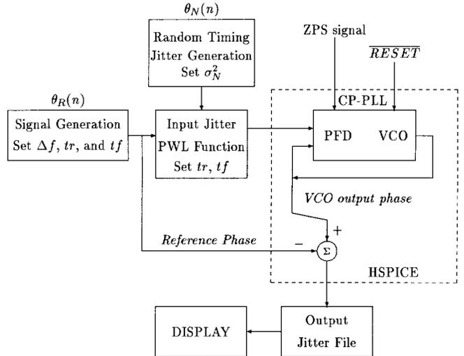
Fig. 13. Simulation setup for the circuit-level model of the optimum gear-shifting CP-PLL.  $\Delta f$ ,  $t_r$ , and  $t_f$  denote the frequency offset, the rising time, and the falling time, respectively.
