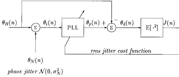
Fig. 2. Block diagram of optimizing scheme for obtaining the optimum gear-shifting sequence of PLL loop gain.
