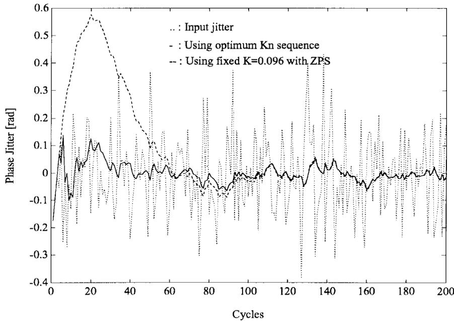
Fig. 9. Real-time phase acquisition using the optimum  $K_n$  sequence and a fixed value of  $K$  ( $=0.096$ ) where  $\sigma_N^2$  and  $\beta$  are  $0.15^2$  and  $0.95$ , respectively.
