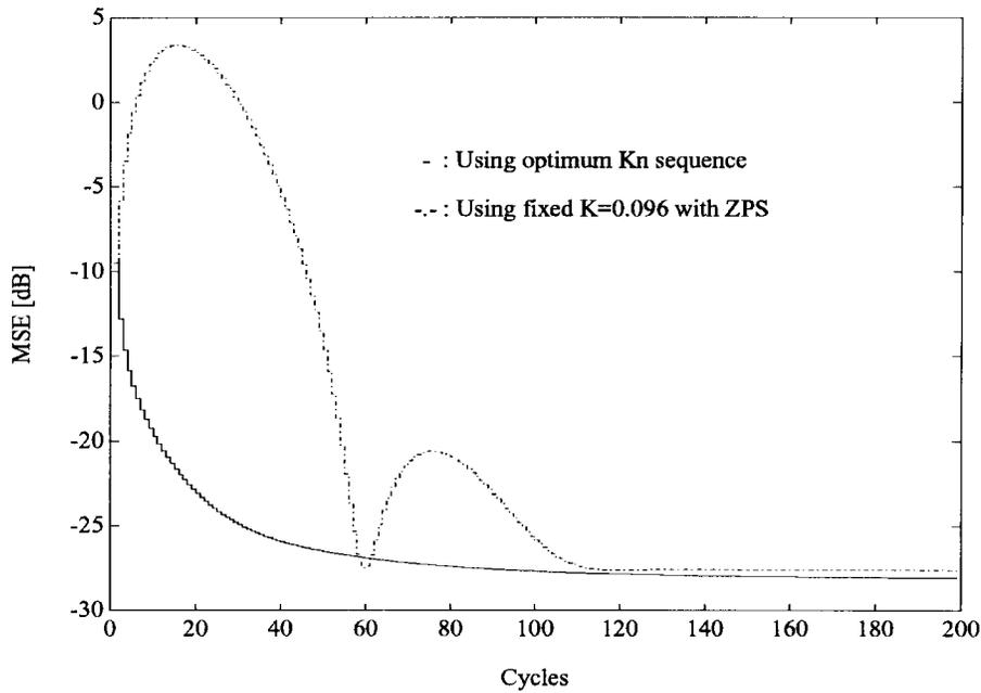
Fig. 8. MSE comparison between the CP-PLL's with the optimum  $K_n$  sequence and a fixed value of  $K$  ( $= 0.096$ ) under conditions of approximately equal MSE in the steady state. Here  $\sigma_N^2 = 0.15^2$  and  $\beta = 0.95$ .
