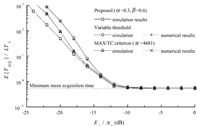
Fig. 3. Performance comparison between proposed and conventional methods in AWGN channel, when  $L = 32767$ .
