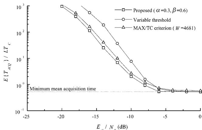
Fig. 4. Performance comparison between proposed and conventional methods in multipath fading channel ( $T_m = 5T_C$ ,  $f_d T_C = 1.0 \times 10^{-4}$ ), when  $L = 32767$ .
