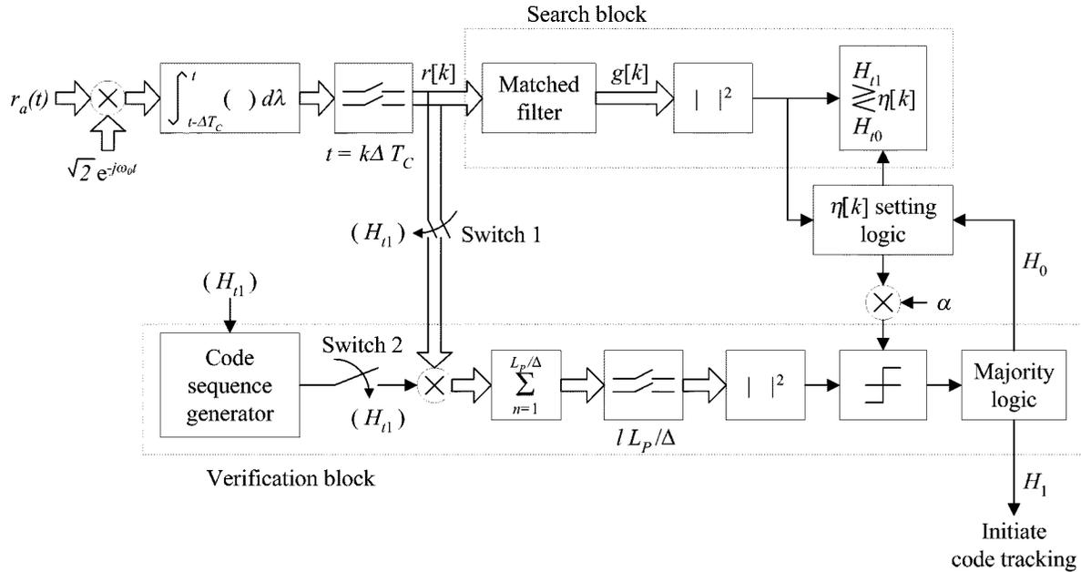
Fig. 1. Proposed code acquisition system.
