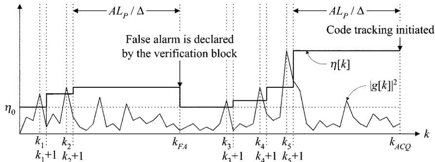
Fig. 2. Typical trajectories of  $\eta[k]$  and  $|g[k]|^2$ . Verification is started at  $k_1$  and  $k_3$ , and it is reset and reinitiated at  $k_2$ ,  $k_4$ , and  $k_5$ .
