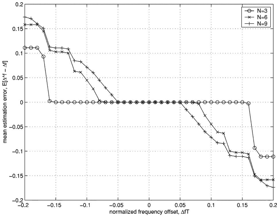
Fig. 3. Mean estimation error (bias) of proposed estimator for fixed ISI channel.
