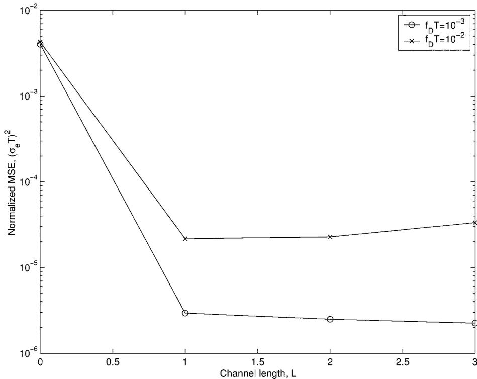
Fig. 7. Sensitivity of the proposed estimator to  $L$  ( $E_b/N_0 = 15$  dB).
