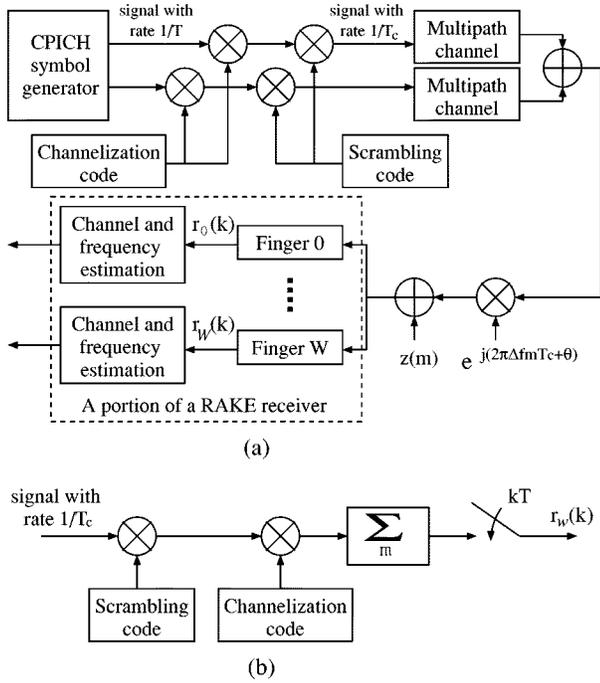
Fig. 12. (a) System model for CPICH of 3GPP where  $T_c$  is chip period. (b) One finger of RAKE receiver in (a).
