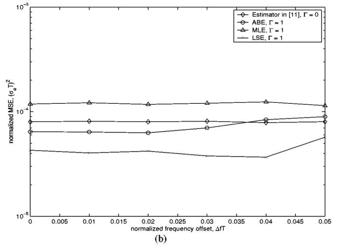
Fig. 14. Performance comparison for transmissions with antenna diversity. (a) Vehicle speed = 3 km/h ( $f_D T = 3.7 \times 10^{-4}$ ) and  $E_b/N_0 = 10$  dB. (b) Vehicle speed = 120 km/h ( $f_D T = 1.5 \times 10^{-2}$ ) and  $E_b/N_0 = 10$  dB.
