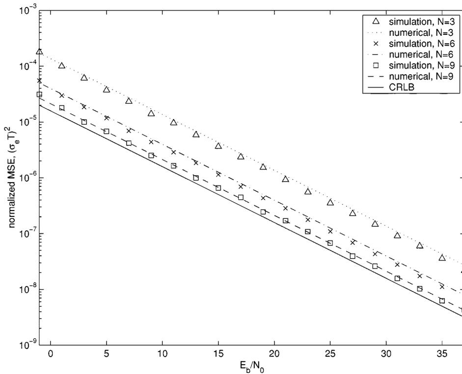
Fig. 4. Normalized MSE of proposed estimator for fixed ISI channel.
