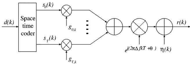
Fig. 11. Baseband system model with transmitter diversity.
