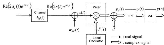
Fig. 1. System employing either direct-conversion or heterodyne architecture.
