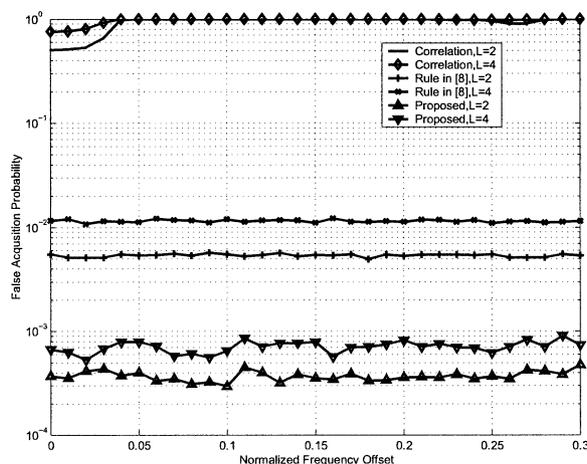
**Fig. 9** Probability of false acquisition for frequency selective channels of length  $L$ .  $E_b/N_0$  was fixed at 24 dB.
