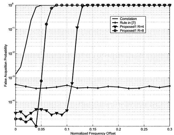
Fig. 6 False acquisition probability vs. normalized frequency offset for AWGN channels when  $E_b/N_o$  is 3 dB.
