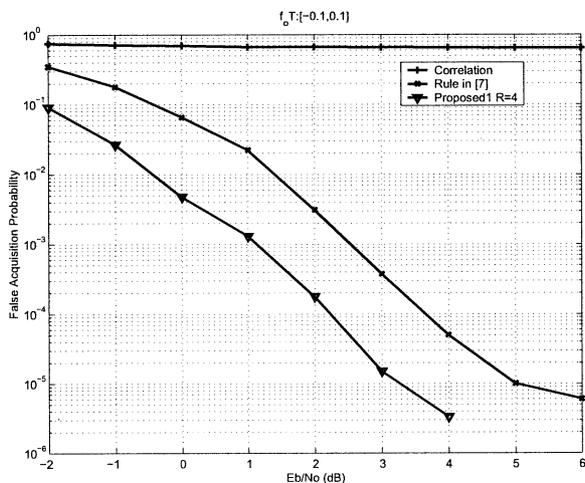
Fig. 5 False acquisition probability vs. signal to noise ratio for AWGN channels.
