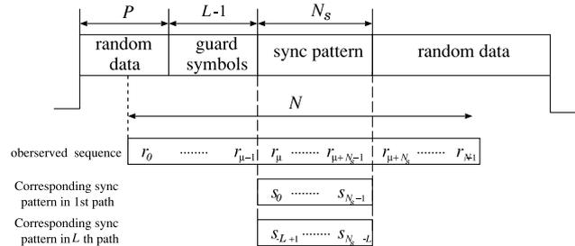
**Fig. 3** Observed sequence and corresponding transmitted data in frequency selective channel, where  $0 \leq \mu \leq P+L-1$ .
