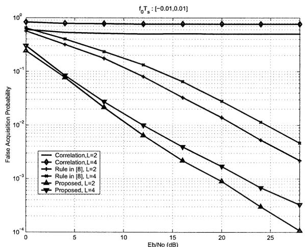
Fig. 7 Probability of false acquisition for frequency selective channels of length  $L$ . The normalized frequency offset was generated randomly over  $[-0.01, 0.01]$ .
