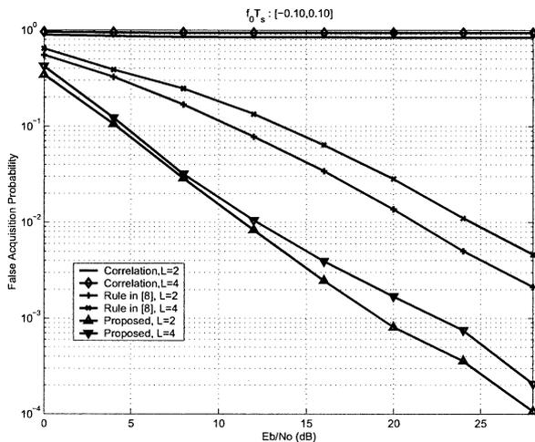
**Fig. 8** Probability of false acquisition for frequency selective channels of length  $L$ . The normalized frequency offset was generated randomly over  $[-0.10, 0.10]$ .
