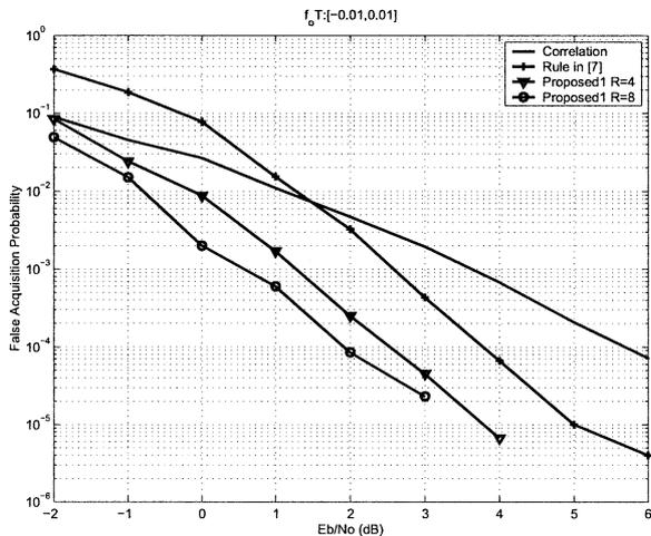
Fig. 4 False acquisition probability vs. signal to noise ratio for AWGN channels.
