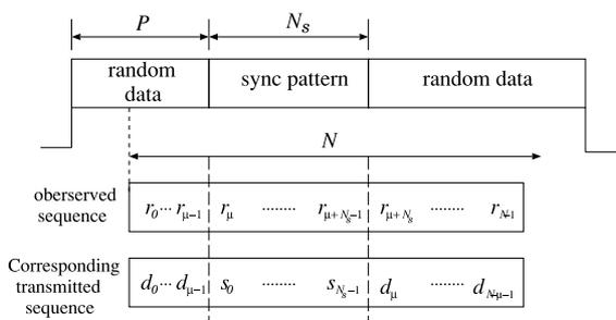
**Fig. 2** Observed sequence and corresponding transmitted data in AWGN channel, where  $0 \leq \mu \leq P$ .
