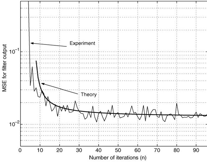
Fig. 4. Learning curves for second equalizer of Algorithm 1 when  $M = 4$ ,  $N = 4$ , and  $E_b/N_0 = 15$  dB.
