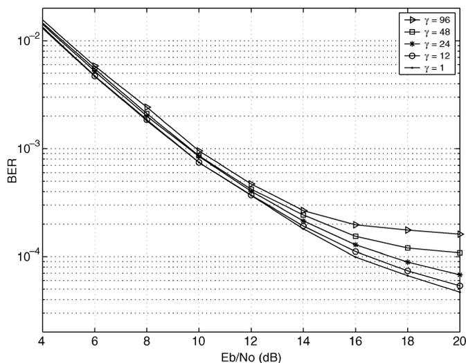
Fig. 8. BER performances of Algorithm 1 and 2 when  $M = 4$ ,  $N = 4$ , and  $f_d T = 0.0005$  (Algorithm 2 becomes Algorithm 1 when  $\gamma = 1$ ).
