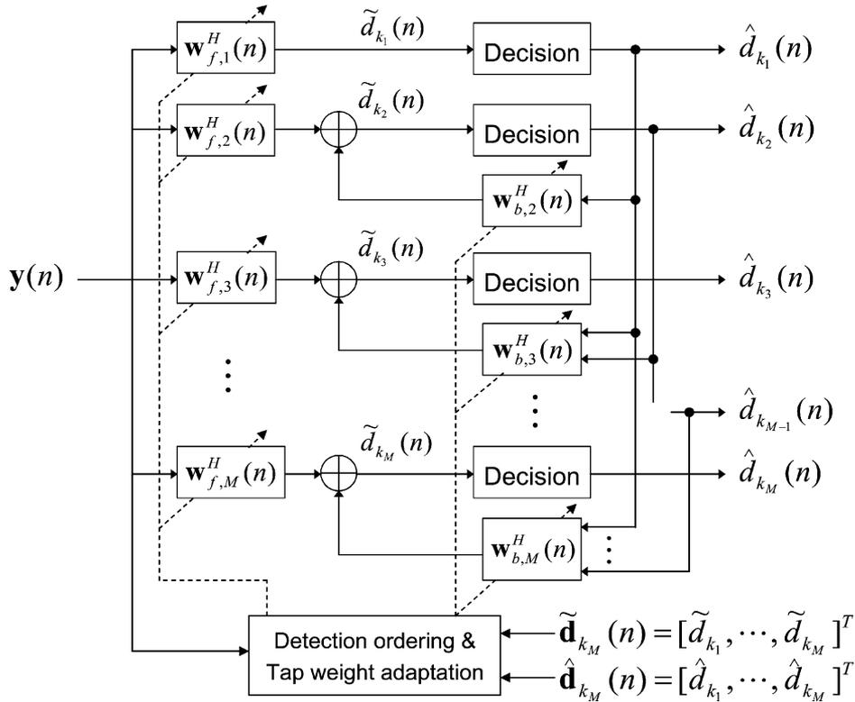
Fig. 2. Detailed architecture of MIMO-DFE.
