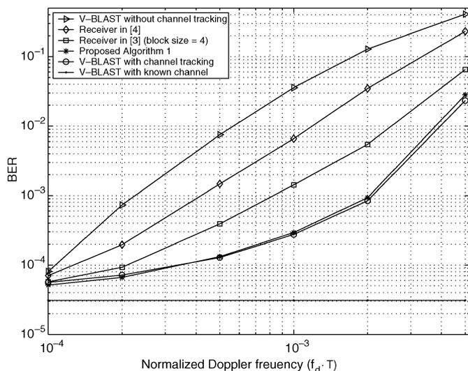
Fig. 7. Comparison of BER performances for various  $f_d T$  values when  $M = 4$ ,  $N = 4$ , and  $E_b/N_0 = 15$  dB.
