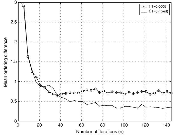
Fig. 5. Mean ordering error curves when  $M = 4$ ,  $N = 4$ , and  $E_b/N_0 = 15$  dB. Here,  $f_d T$  denotes the normalized Doppler frequency.
