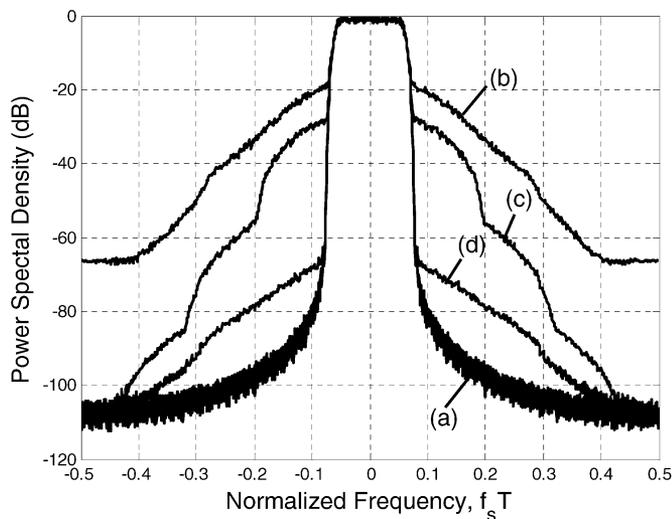
Fig. 3. Power spectral density of the PA output  $y(n)$  when QDM errors exist. (a) Ideal case (PSD of  $s(n)$ ). (b) System employing PD but no QDMC [Fig. 1(a)]. (c) System employing neither PD nor QDMC. (d) Proposed system [Fig. 1(b)].
