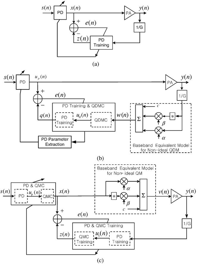
Fig. 1. Baseband equivalent models of a transmitter employing PD with indirect learning. (a) PD when QM and QDM are ideal (no errors). (b) PD when QDM errors exist (ideal QM). (c) Joint PD and QMC when QM errors exist (ideal QDM). Here “\*” denotes complex conjugate.
