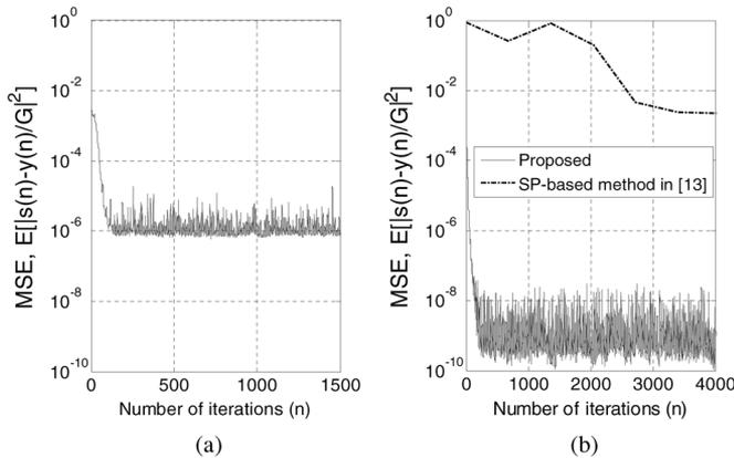
Fig. 2. Learning curves consisting of the MSEs between the input  $s(n)$  and the PA output  $y(n)$  of the proposed systems. (a) PD and QDM error compensation [Fig. 1(b)]. (b) Joint PD and QMC [Fig. 1(c)].
