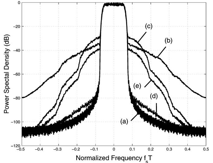
Fig. 4. Power spectral density of the PA output  $y(n)$  when QM errors exist. (a) Ideal case (PSD of  $s(n)$ ). (b) System employing PD but no QMC [Fig. 1(a)]. (c) System employing neither PD nor QMC. (d) Proposed system [Fig. 1(c)]. (e) SP-based method in [13].
