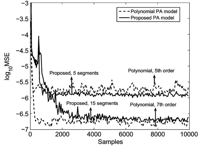
Fig. 5. Learning curves for the proposed and polynomial-based identification schemes. In the proposed scheme, first 500 samples are used for Step 1 and the rest are for Step 2.
