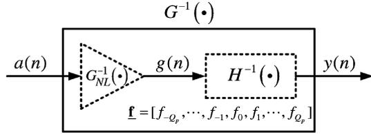
Fig. 4. Inverse of the Wiener model where  $H^{-1}(\cdot)$  is approximated as a noncausal FIR equalizer with impulse response  $\underline{f}$ .
