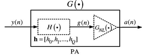
Fig. 2. Wiener system model for a PA with memory.
