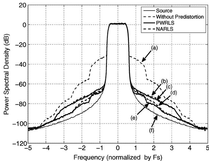
Fig. 7. Comparison of power spectrum density at PA output. (a) Without predistortion. (b) NARLS in [2] with fifth-order polynomial PA model. (c) PWRLS with five segments PA model. (d) NARLS in [2] with seventh-order polynomial PA model. (e) PWRLS with 15 segments PA model. (f) PD input.
