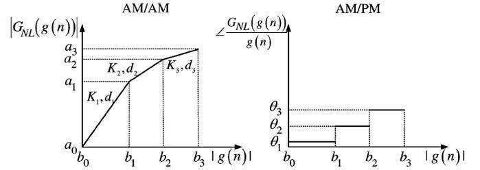
Fig. 3. Piecewise linear model when  $M = 3$ .
