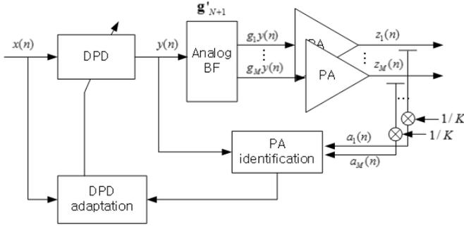
Fig. 2. Digital predistortion structure for an antenna subarray.
