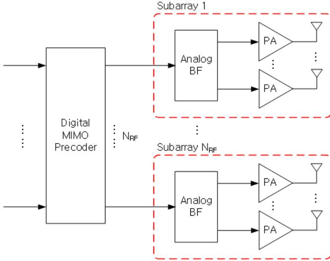
Fig. 1. A hybrid MIMO system with antenna subarrays. Here  $N_{RF}$  is the number of RF chains.
