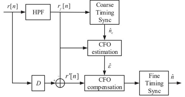
Fig. 4. Proposed synchronization process where  $D$  represents the delay which is equal to the group delay of the high-pass filter (HPF).
