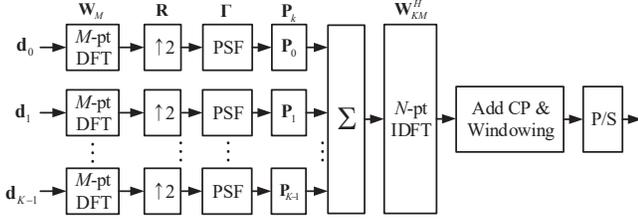
Fig. 1. Structure of a GFDM transmitter.
