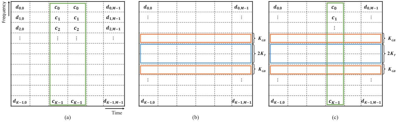
Fig. 2. A GFDM symbol with embedded training sequence. (a) Embedded Midamble. (b) Embedded Training Subcarrier. (c) Hybrid Training.
